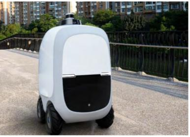
Real-time obstacle detection with the 3D LIDAR sensors. With this feature, the AMR does intelligent path planning and will manoeuvre in a manner to avoid obstacles (humans/objects) • Ultrasonic sensors as a secondary obstacle detection method to stop all motor functions in the event an obstacle is detected within stipulated range (typically 0.5 – 1m in front of
