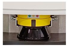
**LASER SCANNER** Detection of obstacles at both the front and rear of the TransCar prevents collisions and accidents in dynamic environments.
